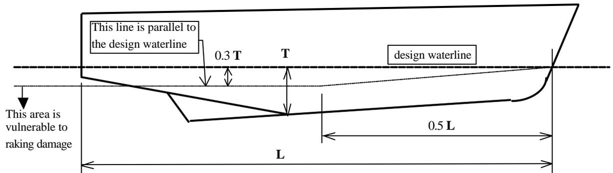
where:  $T$  = maximum draught of the hull (each hull considered individually in the case of multihulls) to the design waterline, excluding any non-buoyant structure
