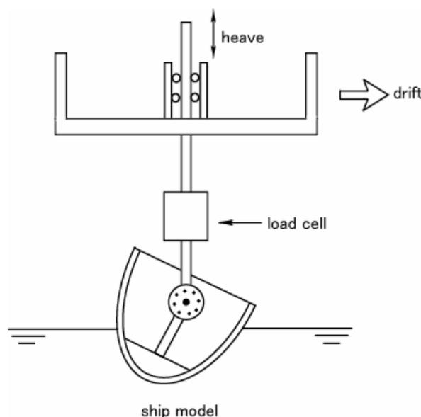
Figure 3.4.1: Example of an arrangement for drifting tests
